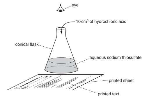
A student used this method to investigate the effect of changing the concentration of the sodium thiosulfate solution on the speed of the reaction.
