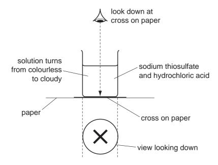
Initially the cross was clearly visible. When the solution became cloudy and the cross could no longer be seen, the clock was stopped and the time recorded.
