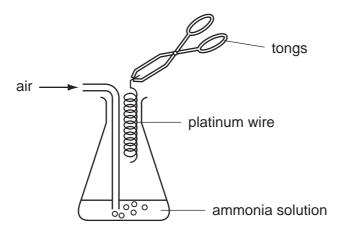
First, nitrogen(II) oxide, NO, is produced. This then reacts with oxygen to form nitrogen(IV) oxide, NO<sub>2</sub>.
