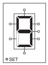
Each of the seven segments of the digital display (currently displaying the number 9) is controlled by its own button which reverses the state of the segment (i.e. turns it on or off) whenever it is pressed. When the SET button is pressed, a number between 1 and 9 inclusive, generated at random, is displayed.
