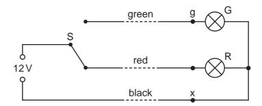
The signal is some way from S to which it is connected by a cable with green, red and black wires. At the signal, the green and red wires are connected to the corresponding lamp and the black wire is connected to a terminal x to provide a common return. The arrangement is shown correctly connected and with the switch set to illuminate the red lamp.
