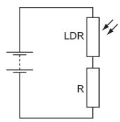
The resistance of the LDR is equal to the resistance of R when no light falls on the LDR.
