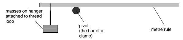
In this situation, the weight  $F_1$  of the masses provides the anticlockwise moment and the weight  $F_2$  of the rule provides the clockwise moment. The weight of the rule acts through the centre of gravity at the middle of the rule. This is shown in the diagram below.
