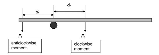
If the rule is balanced, we can apply the principle of moments. This results in the equation
