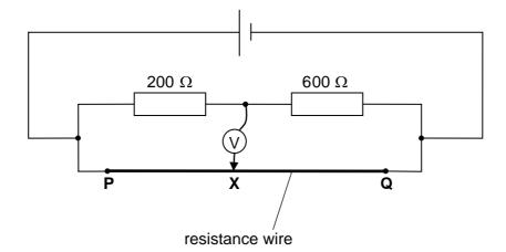
${\bf PQ}$  is a uniform resistance wire of length 100 cm. The position of the contact  ${\bf X}$  is adjusted so that the reading on the voltmeter is zero.
