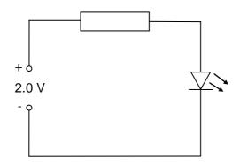
The LED has a working resistance of  $900\Omega$ .
