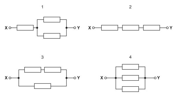
The resistance between **X** and **Y** is measured for each network.
