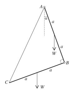
Two uniform rods, *AB* and *BC*, each have length 2*a* and weight *W*. They are smoothly jointed at *B*, and *A* is attached to a smooth fixed pivot. A light inextensible string of length  $(2\sqrt{2})a$  joins *A* to *C* so that angle  $ABC = 90^{\circ}$ . The system hangs in equilibrium, with *AB* making an angle  $\alpha$  with the vertical (see diagram). By taking moments about *A* for the system, or otherwise, show that  $\alpha = 18.4^{\circ}$ , correct to the nearest  $0.1^{\circ}$ . [3]
