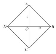
The diagram shows a uniform square lamina ABCD, of mass 4m and with diagonals of length 2a. The diagonals intersect at O. Find the moment of inertia of the lamina about an axis through O perpendicular to its plane.
