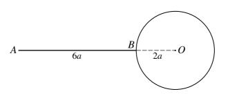
A uniform rod AB, of mass m and length 6a, is rigidly attached at B to a point on the circumference of a uniform circular lamina of mass m, radius 2a and centre O. The lamina and the rod are in the same vertical plane, and ABO is a straight line (see diagram). Show that the moment of inertia of the system about an axis l through A perpendicular to the plane of the lamina is  $78ma^2$ . [4]
