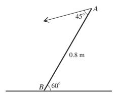
A uniform rod AB has weight 6 N and length 0.8 m. The rod rests in limiting equilibrium with B in contact with a rough horizontal surface and AB inclined at  $60^{\circ}$  to the horizontal. Equilibrium is maintained by a force, in the vertical plane containing AB, acting at A at an angle of  $45^{\circ}$  to AB (see diagram). Calculate
