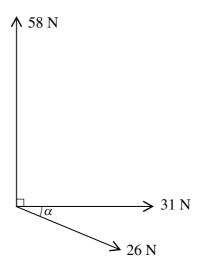
Coplanar forces of magnitudes 58 N, 31 N and 26 N act at a point in the directions shown in the diagram. Given that  $\tan \alpha = \frac{5}{12}$ , find the magnitude and direction of the resultant of the three forces.
