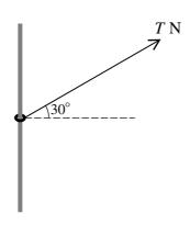
The diagram shows a ring of mass 2 kg threaded on a fixed rough vertical rod. A light string is attached to the ring and is pulled upwards at an angle of  $30^{\circ}$  to the horizontal. The tension in the string is T N. The coefficient of friction between the ring and the rod is 0.24. Find the two values of T for which the ring is in limiting equilibrium.
