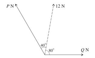
Two forces have magnitudes P N and Q N. The resultant of the two forces has magnitude 12 N and acts in a direction 40° clockwise from the force of magnitude P N and 80° anticlockwise from the force of magnitude Q N (see diagram). Find the value of Q. [4]
