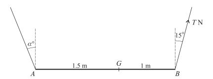
A non-uniform rod AB of length 2.5 m and mass 3 kg has its centre of mass at the point G of the rod, where AG = 1.5 m. The rod hangs horizontally, in equilibrium, from strings attached at A and B. The strings at A and B make angles with the vertical of  $\alpha^{\circ}$  and 15° respectively. The tension in the string at B is T N (see diagram). Find
