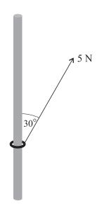
A small ring of mass  $0.6 \,\mathrm{kg}$  is threaded on a rough rod which is fixed vertically. The ring is in equilibrium, acted on by a force of magnitude 5 N pulling upwards at  $30^{\circ}$  to the vertical (see diagram).
