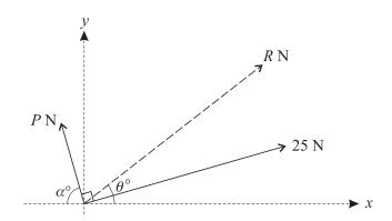
Forces of magnitudes P N and 25 N act at right angles to each other. The resultant of the two forces has magnitude R N and makes an angle of  $\theta^{\circ}$  with the x-axis (see diagram). The force of magnitude P N has components -2.8 N and 9.6 N in the x-direction and the y-direction respectively, and makes an angle of  $\alpha^{\circ}$  with the negative x-axis.
