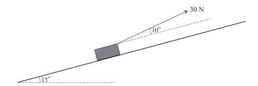
A box of mass 8 kg is pulled, at constant speed, up a straight path which is inclined at an angle of  $15^{\circ}$  to the horizontal. The pulling force is constant, of magnitude 30 N, and acts upwards at an angle of  $10^{\circ}$  from the path (see diagram). The box passes through the points A and B, where AB = 20 m and B is above the level of A. For the motion from A to B, find
