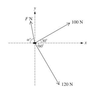
A small box of mass 40 kg is moved along a rough horizontal floor by three men. Two of the men apply horizontal forces of magnitudes 100 N and 120 N, making angles of 30° and 60° respectively with the positive x-direction. The third man applies a horizontal force of magnitude F N making an angle of  $\alpha^{\circ}$  with the negative x-direction (see diagram). The resultant of the three horizontal forces acting on the box is in the positive x-direction and has magnitude 136 N.
