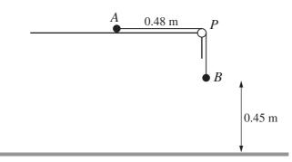
Particle *A* of mass 1.26 kg and particle *B* of mass 0.9 kg are attached to the ends of a light inextensible string. The string passes over a small smooth pulley *P* which is fixed at the edge of a rough horizontal table. *A* is held at rest at a point 0.48 m from *P*, and *B* hangs vertically below *P*, at a height of 0.45 m above the floor (see diagram). The coefficient of friction between *A* and the table is  $\frac{2}{7}$ . *A* is released and the particles start to move.
