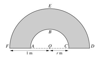
The diagram shows a uniform lamina ABCDEF, formed from a semicircle with centre O and radius 1 m by removing a semicircular part with centre O and radius r m.
