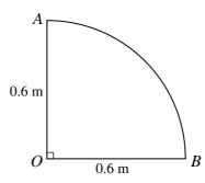
AOB is a uniform lamina in the shape of a quadrant of a circle with centre O and radius  $0.6\,\mathrm{m}$  (see diagram).
