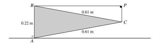
ABC is a uniform triangular lamina of weight 19 N, with AB = 0.22 m and AC = BC = 0.61 m. The plane of the lamina is vertical. A rests on a rough horizontal surface, and AB is vertical. The equilibrium of the lamina is maintained by a light elastic string of natural length 0.7 m which passes over a small smooth peg P and is attached to B and C. The portion of the string attached to B is horizontal, and the portion of the string attached to C is vertical (see diagram).
