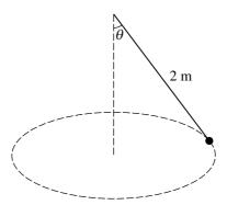
A particle of mass 0.24 kg is attached to one end of a light inextensible string of length 2 m. The other end of the string is attached to a fixed point. The particle moves with constant speed in a horizontal circle. The string makes an angle  $\theta$  with the vertical (see diagram), and the tension in the string is T N. The acceleration of the particle has magnitude 7.5 m s<sup>-2</sup>.
