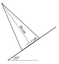
A uniform solid cone has height 30 cm and base radius r cm. The cone is placed with its axis vertical on a rough horizontal plane. The plane is slowly tilted and the cone remains in equilibrium until the angle of inclination of the plane reaches  $35^{\circ}$ , when the cone topples. The diagram shows a cross-section of the cone.
