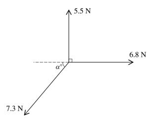
Three coplanar forces act at a point. The magnitudes of the forces are  $5.5 \, \text{N}$ ,  $6.8 \, \text{N}$  and  $7.3 \, \text{N}$ , and the directions in which the forces act are as shown in the diagram. Given that the resultant of the three forces is in the same direction as the force of magnitude  $6.8 \, \text{N}$ , find the value of  $\alpha$  and the magnitude of the resultant.
