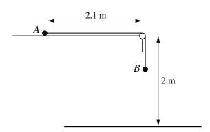
Particles A and B, of masses 0.2 kg and 0.45 kg respectively, are connected by a light inextensible string of length 2.8 m. The string passes over a small smooth pulley at the edge of a rough horizontal surface, which is 2 m above the floor. Particle A is held in contact with the surface at a distance of 2.1 m from the pulley and particle B hangs freely (see diagram). The coefficient of friction between A and the surface is 0.3. Particle A is released and the system begins to move.
