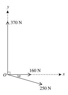
Coplanar forces of magnitudes 250 N, 160 N and 370 N act at a point O in the directions shown in the diagram, where the angle  $\alpha$  is such that  $\sin \alpha = 0.28$  and  $\cos \alpha = 0.96$ . Calculate the magnitude of the resultant of the three forces. Calculate also the angle that the resultant makes with the x-direction.
