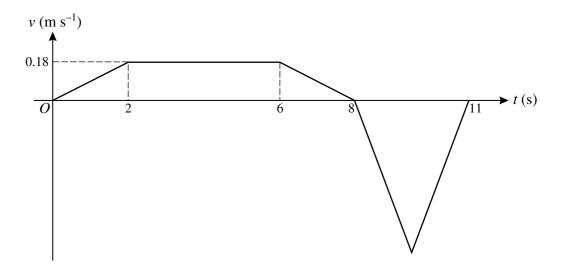
The diagram shows the velocity-time graph for the motion of a machine's cutting tool. The graph consists of five straight line segments. The tool moves forward for 8 s while cutting and then takes 3 s to return to its starting position. Find
