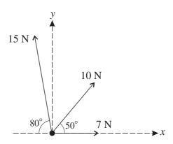
Forces of magnitudes 7 N, 10 N and 15 N act on a particle in the directions shown in the diagram.
