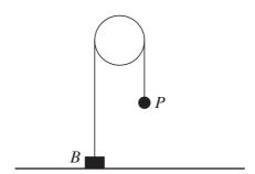
A block B of mass 5 kg is attached to one end of a light inextensible string. A particle P of mass 4 kg is attached to other end of the string. The string passes over a smooth pulley. The system is in equilibrium with the string taut and its straight parts vertical. B is at rest on the ground (see diagram). State the tension in the string and find the force exerted on B by the ground. [3]
