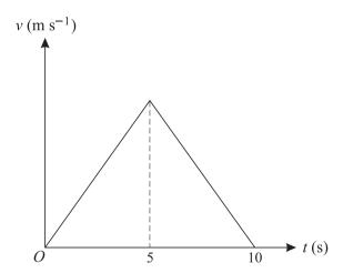
A particle P starts from rest at the point A and travels in a straight line, coming to rest again after 10 s. The velocity-time graph for P consists of two straight line segments (see diagram). A particle Q starts from rest at A at the same instant as P and travels along the same straight line as P. The velocity of Q is given by  $v = 3t - 0.3t^2$  for  $0 \le t \le 10$ . The displacements from A of P and Q are the same when t = 10.
