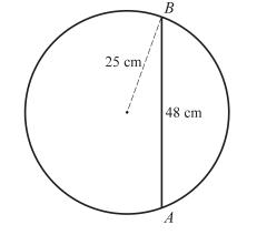
A frame consists of a uniform circular ring of radius 25 cm and mass 1.5 kg, and a uniform rod of length 48 cm and mass 0.6 kg. The ends *A* and *B* of the rod are attached to points on the circumference of the ring, as shown in the diagram. Find the distance of the centre of mass of the frame from the centre of the ring. [4]
