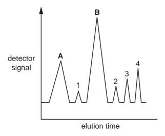
The small peaks 1, 2, 3 and 4 are due to propan-1-ol, ethyl ethanoate, methanol and ethanal, respectively.
