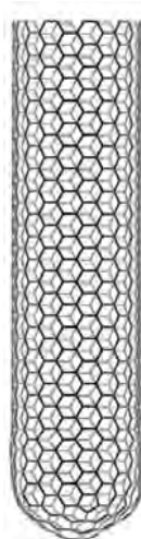
Figure 3.12 – a carbon nanotube closed at one end – a nano “test-tube”
