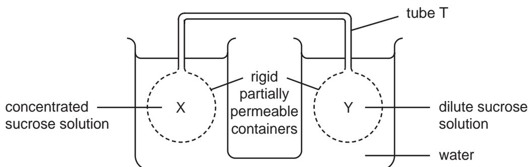
X and Y are filled with sucrose solutions of different concentration, causing water to move in or out of X and Y by osmosis or as a result of hydrostatic pressure. Sucrose solution then moves through the tube T joining X and Y.
