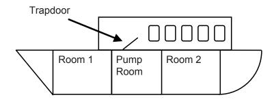
If water is present in either Room 1 or Room 2, and the trapdoor to the pump room is closed, the pump automatically starts working.
