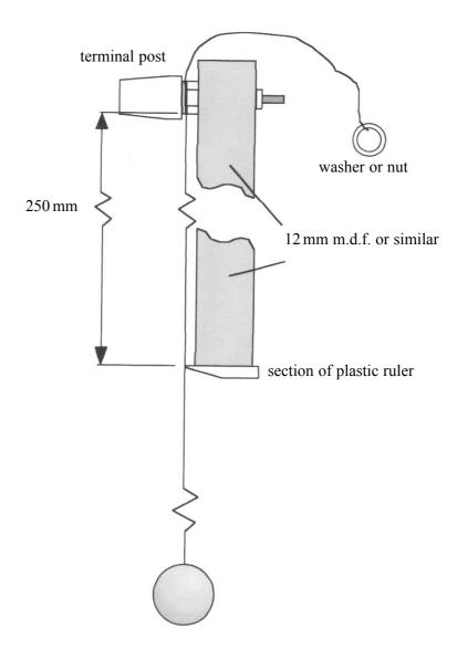
Clamp the m.d.f. so that the pendulum overhangs the edge of the bench. The terminal post should be about 100 mm above the top of the bench. Adjust the length of the pendulum so that the bob hangs freely about 100 mm above the floor and when the thread is at rest and hanging vertically it just touches the protruding edge of the ruler.
