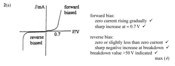
(b) forward bias: high resistance (initially gives small current)  $\checkmark$ at  $\approx 0.7$  V, resistance decreases rapidly (current increases)  $\checkmark$
