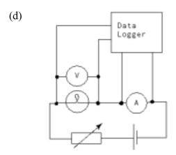
variable supply or rheostat, (in series with filament) or pot. divider ✓ filament and current sensor in series ✓ voltage sensor across filament ✓ connections to datalogger ✓
