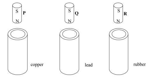
Three vertical tubes, made from copper, lead and rubber respectively, have identical dimensions. Identical, strong, cylindrical magnets P, Q and R are released simultaneously from the same distance above each tube. Because of electromagnetic effects, the magnets emerge from the bottom of the tubes at different times.
