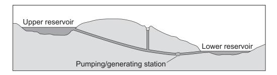
At night, when power stations across the country are producing more electricity than is needed, excess electricity is used to pump water uphill from the lower reservoir to the upper reservoir.
